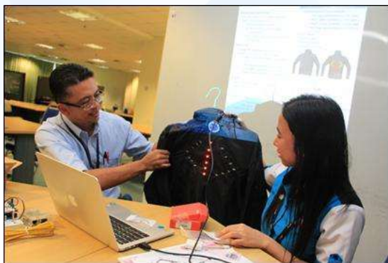
Principle Investigator, Dr Johari Abdullah and project member, Kho Kai Li are testing the CycleSense solution, a sensor-based bicycle safety system.
